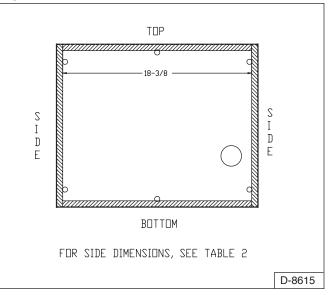
Figure 4 - Horizontal Vent Termination Location
